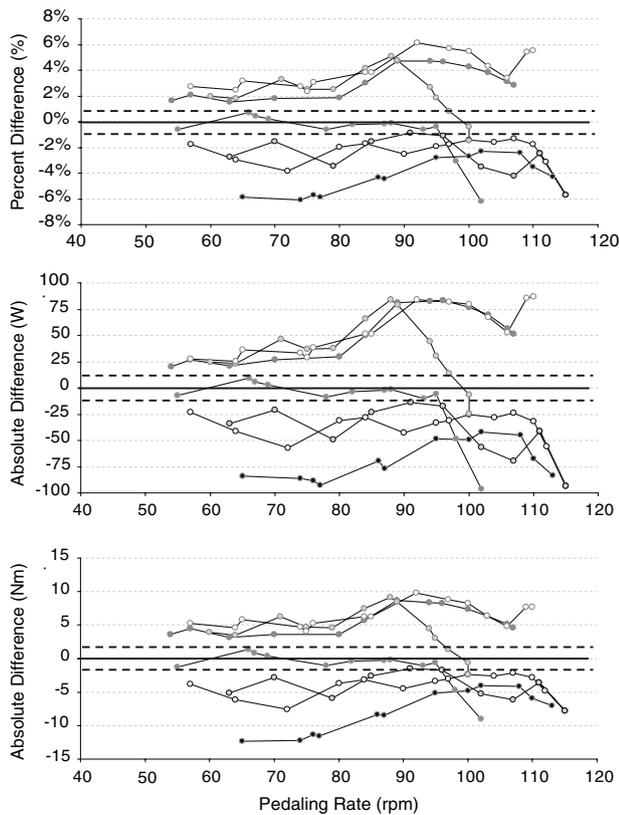
**Fig. 3** Modified Bland-Altman plots of absolute torque (below), absolute power (middle) and error % of predicted power (matched for pedaling rate from laboratory-derived regression coefficients) from actual data measured in the field. The mean error % ( $\pm$ SD) for all participants ( $n = 7$ ) was  $0.1 \pm 3.3$  %. The dotted lines represent the 95% CI. The plot shows the individual variation between laboratory and field torque and power
