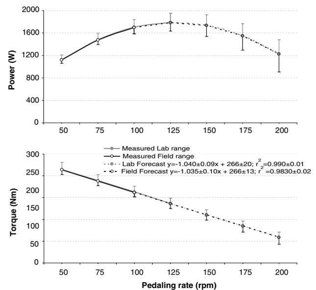
**Fig. 2** Graph of mean ( $\pm$ SD) torque-pedaling rate regression equations and power-pedaling rate relationships for laboratory and field tests. The linear equations represent the average slope and y-intercepts for all participants ( $n = 7$ ). The *solid lines* represent the measured range of data and the *dotted lines* show the forecast relationship. The average fit of all seven regression equations ( $r^2$ ) is presented with the equations
